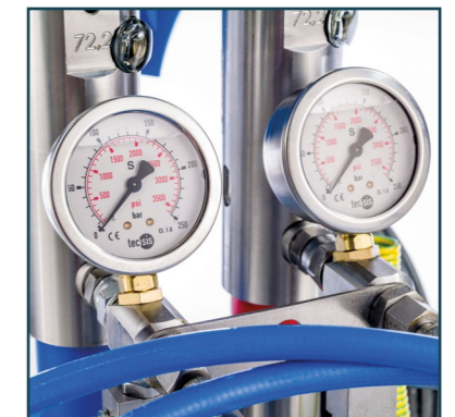
Readable injection pressures for both components
