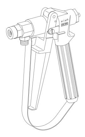
CAUTION! Handle gun with care - Nozzle The WIWA-Airless gun, model WIWA 500 F, has been designed to withstand operating pressures of 500 bar.
